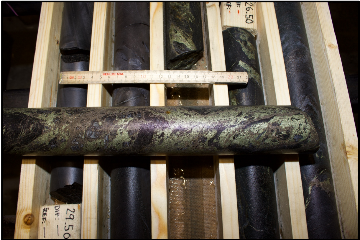
Figure 4. Close-up image of the mineralized drill core. The semi-massive sulphide mineralization (bronze colours) hosts nickel and copper and cobalt
