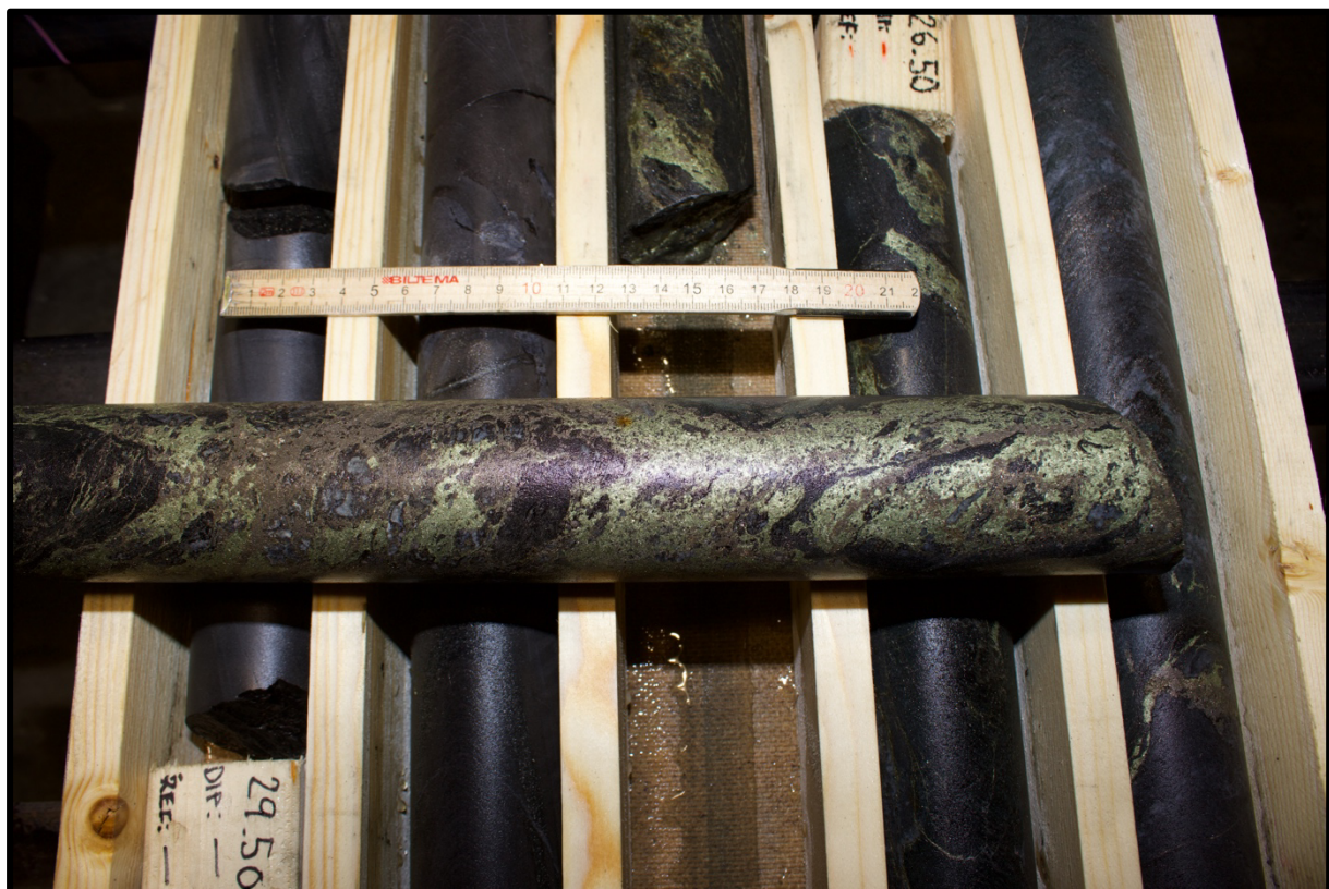
Figure 2. Close-up image of the mineralized drill core. The semi-massive sulphide mineralization (bronze colours) hosts nickel and copper
