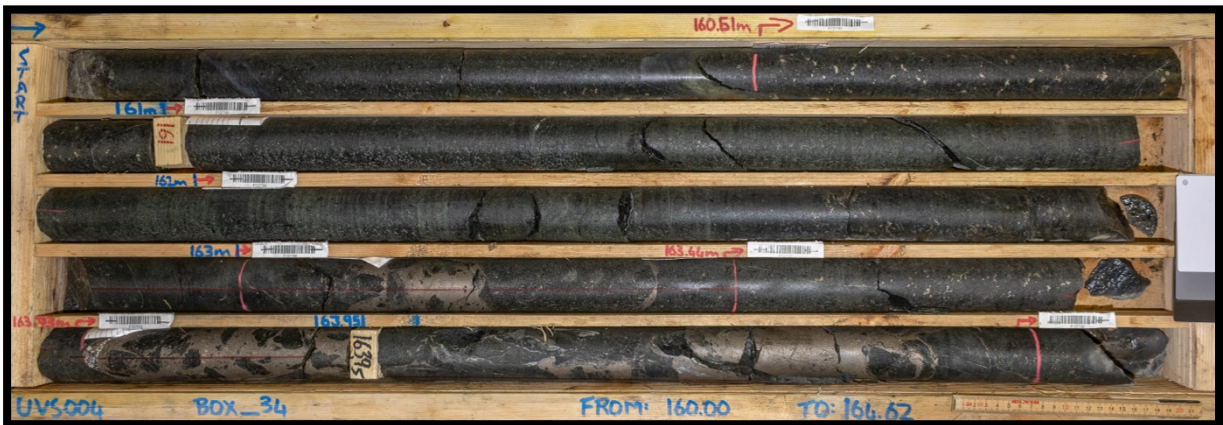
Figure 3. Top: core photo of UVS_002 with 0.9 m @ 1.6% Ni, 0.17% Cu, 0.85% Co & 1.1 g/t 3PGE (3.29% NiEq*). Bottom: core photo of UVS_004 with 0.8 m @ 1.0% Ni, 0.42% Cu & 0.09% Co (1.29% NiEq*)
